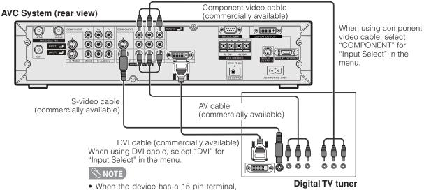
When the device has a 15-pin terminal, use a commercially available D-sub cable to connect it.
